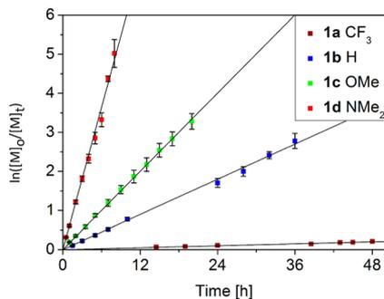
**Figure 3.** Kinetic analysis of the polymerization reaction according to a (pseudo) first-order rate law (lines show the linear fits).
