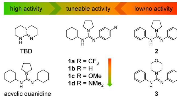
**Figure 1.** Guanidine organocatalysts for polymerization of lactide.
