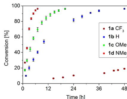
**Figure 2.** Monomer conversion vs time for ROP of *L*-lactide catalyzed by **1a**–**1d** with  $M/I/C$  ratio = 50:1:1. Experiments performed in triplicate (error bars represent standard deviation).
