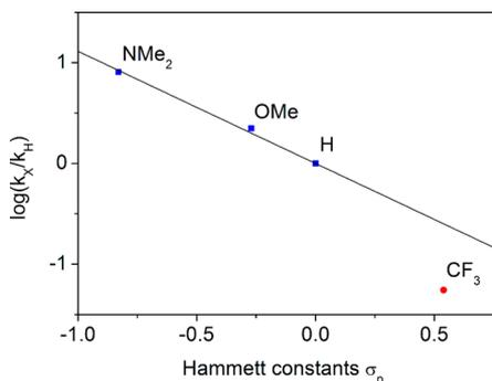
**Figure 4.** Application of the Hammett equation to the rate constants  $k_{app}$  and the respective Hammett constants  $\sigma_p$  of the substituents. $^{18}$
