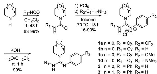
pyrrolidine and morpholine with cyclohexyl or phenyl isocyanate, respectively. Subsequently, the formed carbamides were transformed to their Vilsmeier salts, which were reacted *in situ* with the different aniline derivatives to give the guanidine hydrochlorides. In the final step, the hydrochlorides were exposed to a potassium hydroxide solution to obtain the free guanidines **1**–**3** quantitatively.
