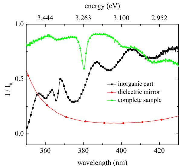
FIG. 2. Transmission of the inorganic cavity part (black squares,  $T = 77$  K), the dielectric top mirror on a reference sample (red circles,  $T = 300$  K), and reflection spectrum of the whole structure (green triangles,  $T = 5$  K).
