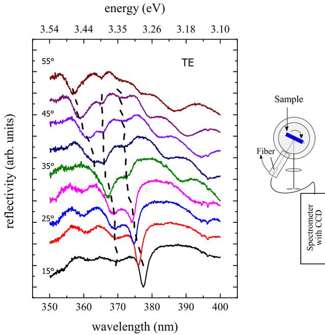
FIG. 3. Left: Angular-resolved reflectivity spectra measured with TE polarized light at 5 K (horizontally shifted for clarity). Dashed lines give the reflection minima corresponding to the polariton resonances for the whole set of spectra. Right: Measuring geometry used.
