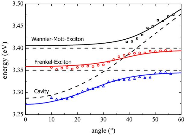
FIG. 4. Angular dependence of the energetic position of the reflection minima. Symbols: experimental reflection minima, lines: fits by the oscillator model with  $V_{LAP} = 27$  meV,  $V_{ZnO} = 24$  meV,  $n_{\text{eff}} = 2.66$ , and  $\hbar\omega_c(0) = 3.29$  eV. The undisturbed excitonic resonances and the cavity dispersion are shown by the dashed lines.
