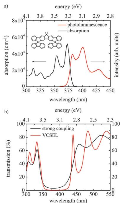
**Figure 1.** Components of the microcavities: a) Absorption and emission spectra of L4P-Sp2 in a polymer matrix. Inset: Structural formula of the molecule. b) Transmission spectra of the  $\text{ZrO}_x/\text{SiO}_x$  mirror stacks for strong coupling (black) and VCSEL (red).
