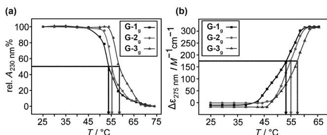
Figure 1. a) UV/Vis and b) CD spectral evolution as a function of temperature to determine the LCST for **G-n<sub>g</sub>** ( $c = 8.5 \cdot 10^{-6} \text{ M}$ ).
