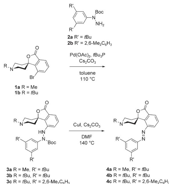
**Scheme 1.** Modular synthesis spirofused piperidines **4a–c** with variable steric demand by a two-step sequence of Pd-catalyzed cross-coupling followed by oxidation. Boc = *tert*-butoxycarbonyl, DMF = *N,N*-dimethylformamide.
